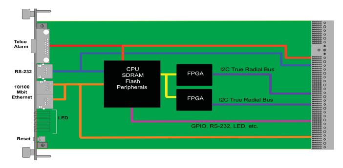
FIGURE 2. VT008 Functional Block Diagram
